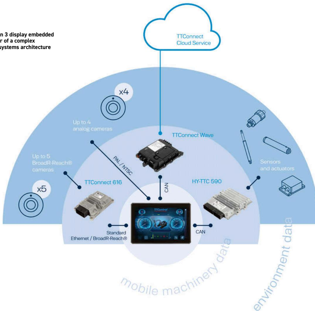
features, bringing about entirely new use-cases and business models. TTControl's Vision 3 display series and its set of interfaces combined with TTControl's IoT platform TTConnect Cloud Service prepares mobile machinery for the next level of connectivity.
