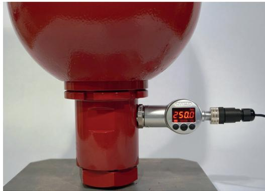
Recommended installation with a bladder accumulator (at the vent screw of the oil valve)
